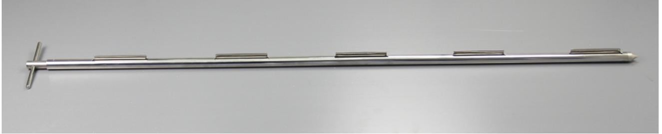
Outer Diameter of Outer Tube: 25 mm (plus 10mm approx.. for scrapers)
