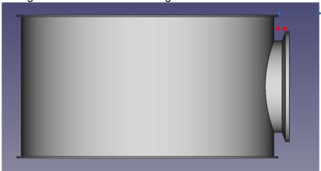
Mount the sampler to this triclamp flange using the clamp band and seal. Connect the air supply pipes to the appropriate fittings (6 + 7). **Air pressure**: 0,8-1,2bar Connect the sample container or system onto the sample outlet spout (9). Adjust air throttle to limit speed of the cup movement. (0,2 m/s)
